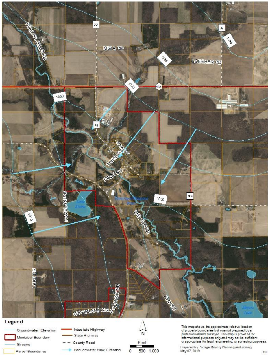
Figure 2. Approximate groundwater flow direction into the Village of Nelsonville based on groundwater elevation.
